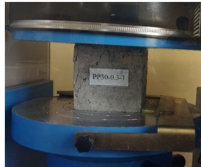
Fig. 3. Appearance of polypropylene fiber-based fiber concrete after testing. Photo taken by Asalxon Juraeva at the Namangan State Technical University Laboratory June 2025
