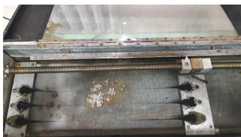
Fig. 2. Stretchability characteristic of polymer-sulfur bitumen with a sulfur content of 20 %
