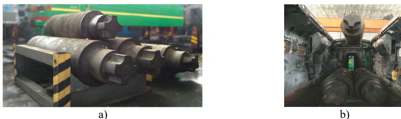
Fig. 3. Implementation of the testing process: a) test loads of different weights; b) placement of the loads onto the locomotive frame using a crane
