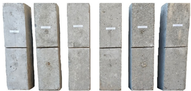
Fig. 3. Concrete prism specimens with added combination of steel and basalt fibers. Photo taken by Bakhtiyor Maksud Ugli at the Namangan State Technical University Laboratory, April 2025
