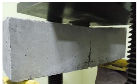
Fig. 6. General view of the sample after the test: a) ordinary concrete and b) fiber concrete. Photo taken by Bakhtiyor Maksud Ugli at the Namangan State Technical University Laboratory, April 2025
