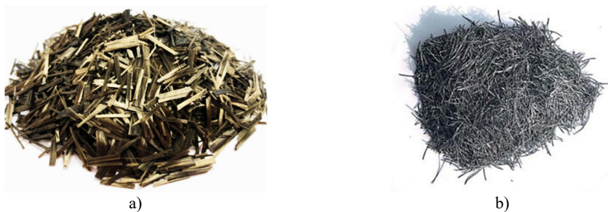
Fig. 2. Appearance of a) Basalt, b) steel fibers. Photo taken by Bakhtiyor Maksud Ugli at the Namangan State Technical University Laboratory, March 2025
