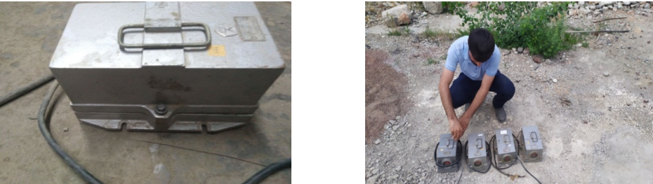
Fig. 6. Vibrations detectors that consider the key parameters of the vibrations on the railway roadbed in 3-axis coordinate system (x, y, z) . The photograph, taken by the second author on May 19, 2022, provides a general view of seismometric sensors that record the process of vibrations in the earth’s surface
