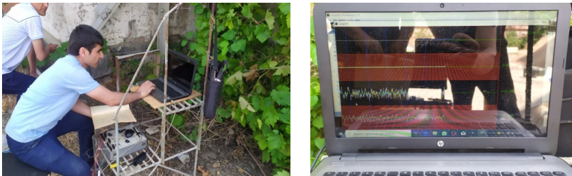
Fig. 8. The recording vibrations that take place in the railway roadbed using SM-3 sensors on the computer. The photograph taken by the second author on May 19, 2022, shows the process of recording ground vibrations using a computer program
