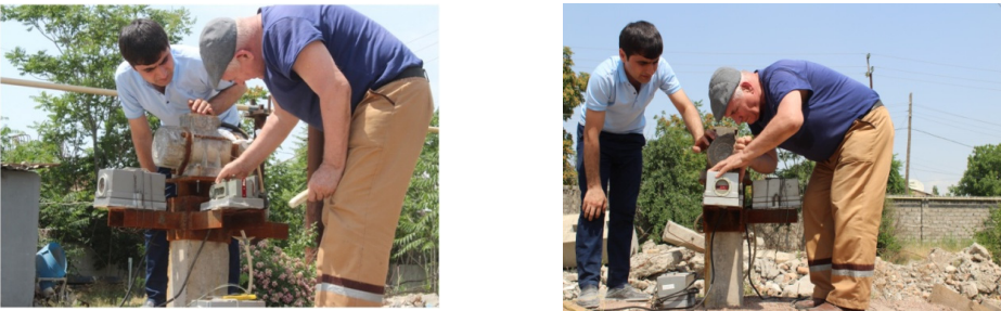
Fig. 7. The SM-3 sensors and a vibrator on railroad roadbed in three-axis coordinate system (x, y, z) .
