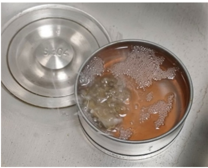
Fig. 4. Oil quenching process. Photo taken by M.Z. Ubaydullaev (co-author) in the laboratory of the Almalyk Branch of NUST MISIS, 2025)
