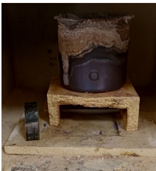
Fig. 2. Sample and steel crucible in the muffle furnace. Photo taken by M.Z. Ubaydullaev (co-author) in the laboratory of the Almalyk Branch of NUST MISIS, 2025
