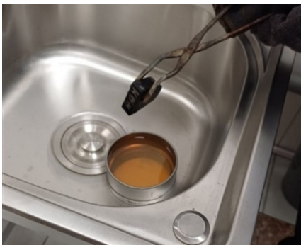
Fig. 4. Oil quenching process. Photo taken by M.Z. Ubaydullaev (co-author) in the laboratory of the Almalyk Branch of NUST MISIS, 2025)
