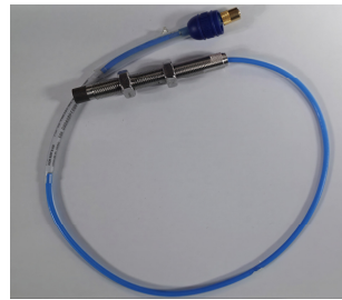
b) Proximity probe using Eddy currents
