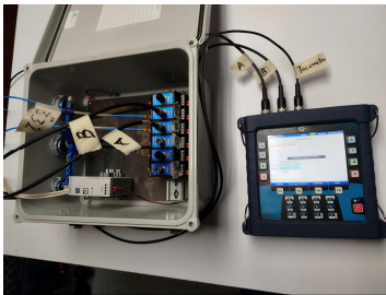
a) DSP logger expert vibration measurement equipment
