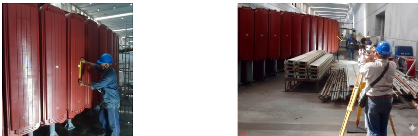
Fig. 15. Measurement of magnetic center of rotor [12]. Photographs were taken at the unit under study by P. Hernandez on December 13, 2022.
