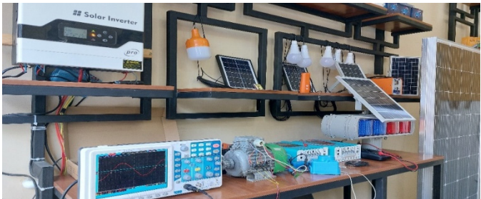
Fig. 3. Research experiment process of an asynchronous motor electromagnetic converter powered by a single-phase power grid powered by solar panels. The photograph was taken by S. Azamov on 18 October 2024 in the Electrical Engineering Department Laboratory of Andijan State Technical Institute
