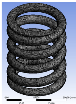
Fig. 2. Imported spring geometry and visual inspection of mesh uniformity
