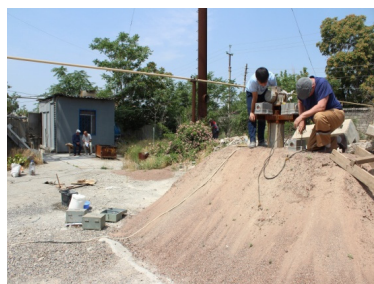
Fig. 2. Location of measurement points with seismometers. In the photograph taken by the first author on May 19, 2022, a model of the earthwork prepared by the author is shown, and the process of vibrations was recorded
