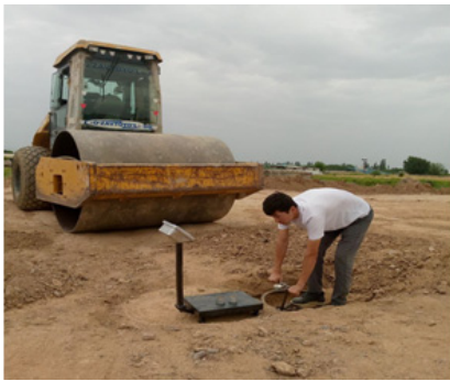
Fig. 3. Determination of strength indicators using a single-plane circular chisel. The figure shows the DU-62 vibratory roller
