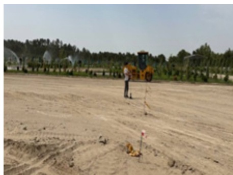
Fig. 2. Determination of the calculated parameters of sandy soils in the field before the effect of vibration
