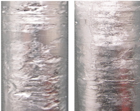
Fig. 2. Surface quality of control and experimental blanks made of AD35 alloy. The photograph was first taken by Uzdieva N.S. and Vakhidova K.L. in 2019 at the “Nanotechnology and Nanomaterials” Collective Use Research Center of the Groznian State Oil Technical University
