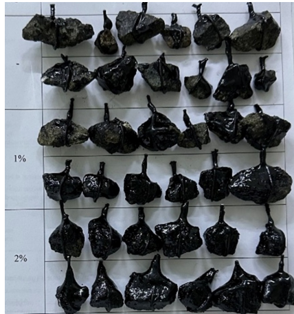
Fig. 8. Adhesion of crushed stone with the addition of 1% and 2% “TITAN” modifiers to bitumen and with ordinary BND 90/60 grade bitumen
