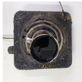
b) Bitumen heating
