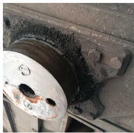
b) Central support pivot crack
