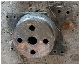
a) Fracture of central support pivot
