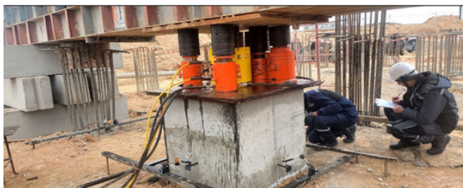
Fig. 4. An image of the indicators that were put up to track the testing pile's movement while it was being tested and the process of taking counts from them. Photo taken by the author at the Tebinbulok site on December 15, 2023
