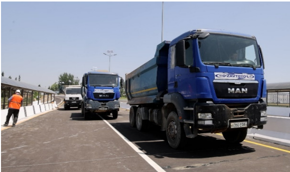
Fig. 3. Static truck-load test setup for determining actual load-carrying capacity (M-41 highway, Andijan region, 15 May 2025; photo by first author)
