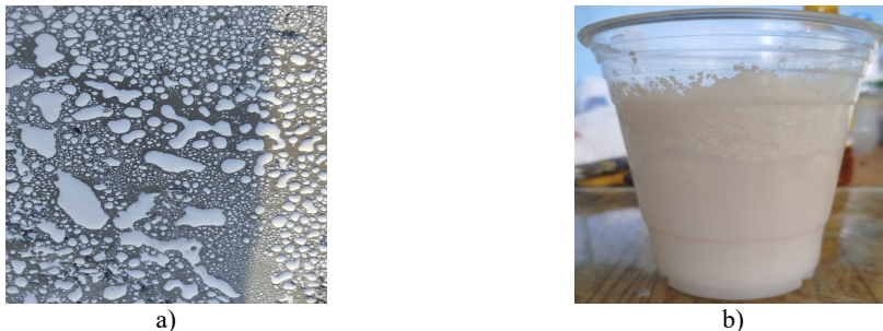
Fig. 4. Verification of film-forming materials: a) type of film-forming material with expired shelf life, sprayed on the surface of freshly laid cement concrete; b) separation of film-forming material and formation of particles larger than 1 mm. Photograph taken by Tukhtayev Matchon Bekjonovich in the laboratory and on field test sections of newly constructed cement concrete pavement, Tashkent, Uzbekistan
