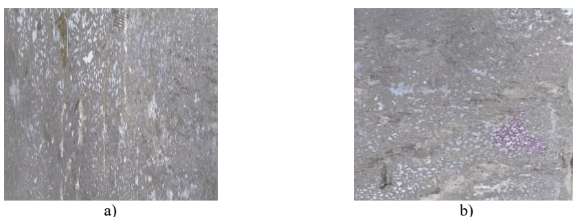
Fig. 3. Testing film-forming materials: a) testing the film-forming material with a 10 % solution of hydrochloric acid; b) testing the film-forming material with a 1 % solution of phenolphthalein. Photograph taken by Tukhtayev Matchon Bekjonovich in the laboratory and on field test sections of newly constructed cement concrete pavement, Tashkent, Uzbekistan
