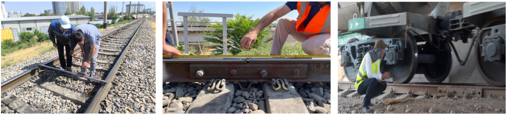
Fig. 2. Inspection of bridge transition and rail joint zones as the main object of the study. The photograph, taken by the third author during research conducted in 2024-2025, depicts the processes of measuring and monitoring the railway bridge transition and rail joint zones using the SUP-3 track gauge template
