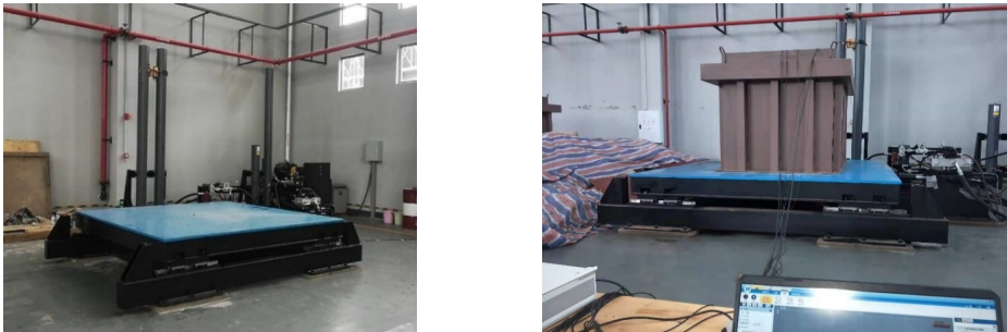
a) Shaking table b) Loading system Fig. 2. Shaking table and loading system. Image credit: Xukai Tan, State Key Laboratory of Mountain Bridge and Tunnel Engineering, 2025
