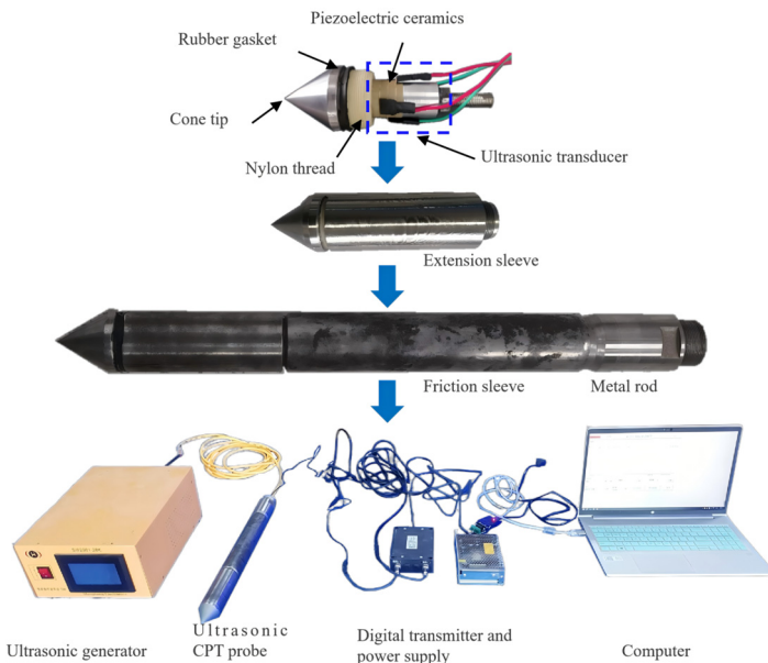
Fig. 2. Structure of the ultrasonic CPT probe. The photos were taken by Zhehong Shen at Shaoxing University on October 23, 2024
