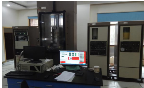
Fig. 2. MTS 815 Electro-hydraulic Servo-controlled Rock Triaxial Testing System. Photo by Haijie Wen, Zhuzhou, China, July 16, 2025
