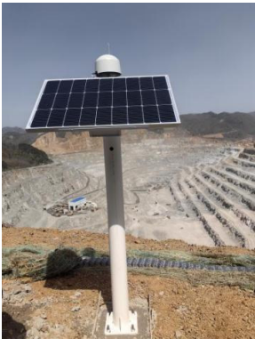
Fig. 11. GNSS Monitoring Points. Photo by Jia Haipeng in July 2024 on the south slope of the Longyu Large Open-Pit Mine
