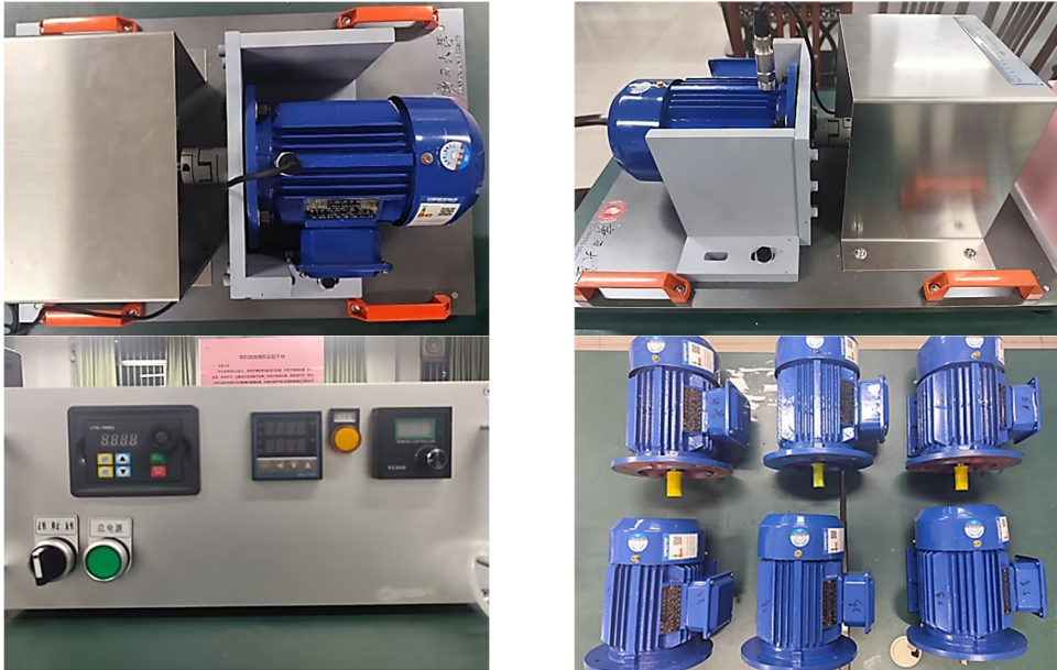
Fig. 5. GXU motor multi-type fault data acquisition experimental platform.
