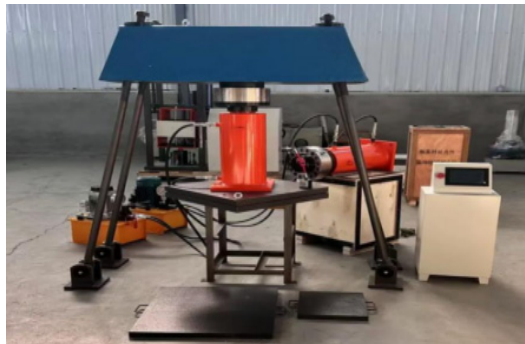
Fig. 12. In-Situ direct shear apparatus. Photo by Jia Haipeng in 2025 at the Rock Mechanics Laboratory, School of Intelligent Construction, Henan University of Urban Construction
