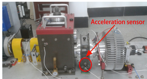
Fig. 4. Installation location of acceleration sensor. Photo by authors in Tiangong University, Tianjin, China, 2024
