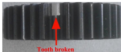
Fig. 6. One tooth breakage of fixed-axle gear. Photo by authors at Tiangong University, Tianjin, China, 2024
