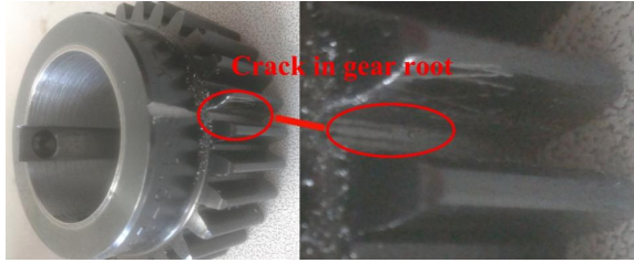
Fig. 9. Fixed-axle gear crack on root of tooth. Photographed at Tiangong University, Tianjin, China, 2024
