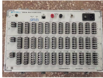
b) Strain gauge demodulation equipment
