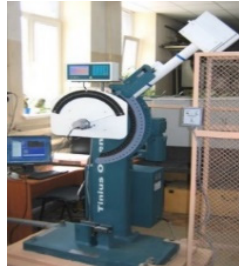
Fig. 1. General view and functional components of the experimental test stand designed for dynamic impact loading. Photo by N. Muhammadiev at TSTU laboratory, May 2025
