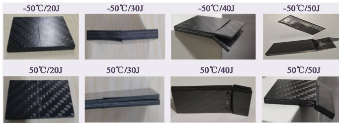
Fig. 7. Damage morphology. Photo by Fengfeng Wang, Composite Material Testing Lab of Jingling Institute of Technology, 2025
