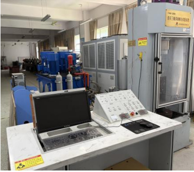
Fig. 5. Rock triaxial multi-field coupling experimental system
