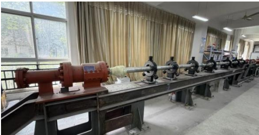
Fig. 10. Device diagram of SHPB experimental system
