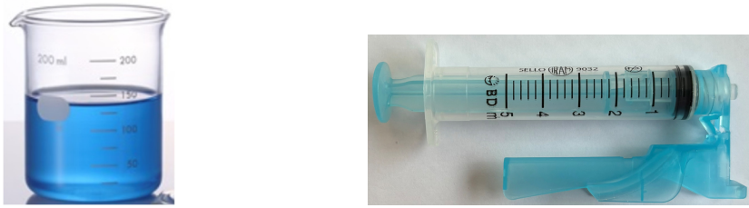
Fig. 5. Becker and syringe used to measure the resin volume
