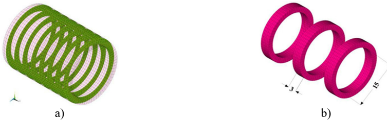
Fig. 4. Option No. 1: a) finite element approximation of deformation joints and b) thickened lining sections
