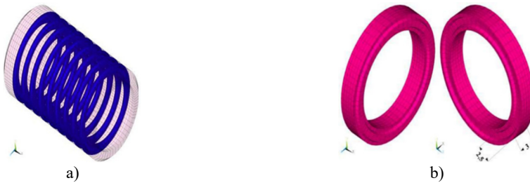
Fig. 5. Option No. 2. Three-dimensional finite element approximation of the Tunnel No. 3 – enclosing rock mass system in the Ionakhsh Fault zone: 1 – sandstone; 2 – crushing zone; 3 – friction clay; 4 – argillites; 5 – standard tunnel lining; 6 – thickened lining with grooved joints
