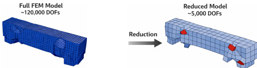
Fig. 3. Illustration of the Guyan model order reduction: a) full finite element model and b) reduced order model, retaining dominant vibration modes
