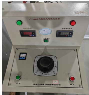
Fig. 2. High-current generator. The original photograph was taken by Guangmin Gu at the High-Voltage Laboratory, Nanjing Institute of Technology, Nanjing, Jiangsu, China, on November 20, 2025
