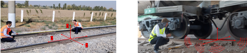
Fig. 1. Propagation of vibrations through the track elements resulting from the interaction between the wheelsets and the rail. The photograph was taken during research conducted by the second author in 2024-2025 and illustrates the process of studying issues in the rail joint zones of the railway track
