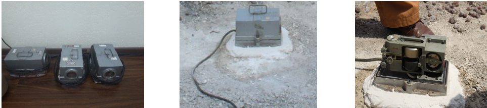
Fig. 3. Sensors for determining the main parameters of oscillations in three main coordinate systems x , y , z . Photos by the second author in the process of determining the amplitude-frequency characteristics of oscillations as a result of train movement in the zone of railway track joints in a photograph taken on December 10, 2025
