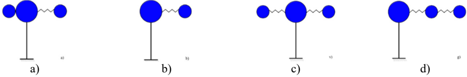
Fig. 2. Calculation schemes of span structures in various connections with supports: a) seismic protection + rigid support part; b) seismic protection + movable support part; c) seismic protection + seismic protection; d) seismic protection + spring + movable support part
