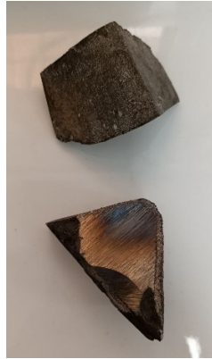
Fig. 1. 35KhML steel samples with and without the addition of the modifier.
