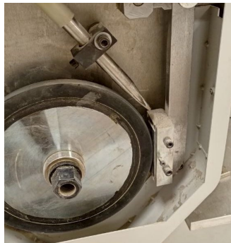
Fig. 2. Wear resistance tests using the Brinell-Haworth method.
