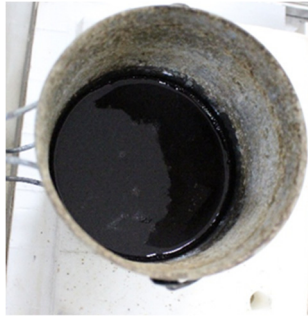
Fig. 3. Immersion of specimens into the molten salt bath. Photo by the authors in the laboratory of the Almalyk Branch of NUST MISIS 2026
