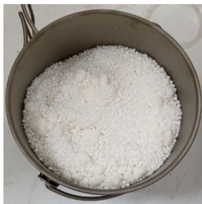
Fig. 1. Loading of urea and potash (600 g) into the titanium crucible. Photo by the authors in the laboratory of the Almalysk Branch of NUST MISIS 2026
