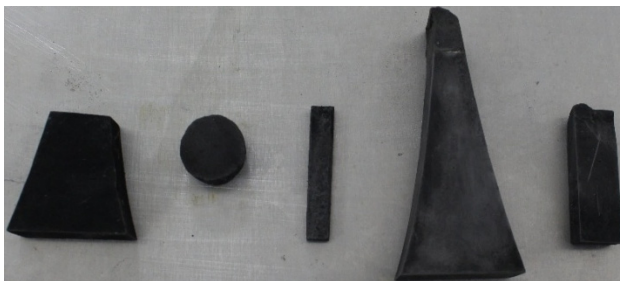
Fig. 5. Carbonitrided specimens. Photo by the authors in the laboratory of the Almalyk Branch of NUST MISIS 2026
