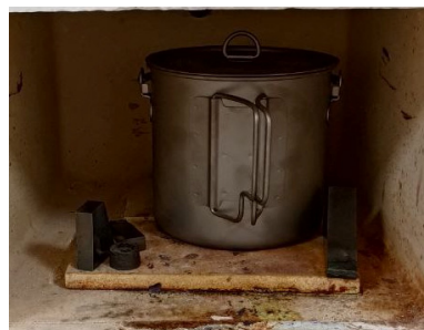
Fig. 2. Heating process of salts and specimens in the muffle furnace. Photo by the authors in the laboratory of the Almalysk Branch of NUST MISIS 2026
