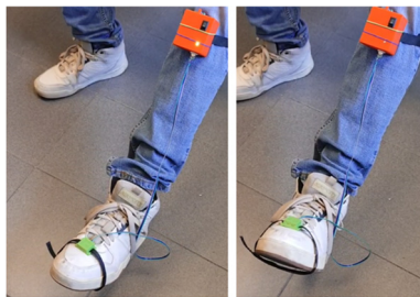
Fig. 7. Snapshot of the experiment with the device worn by the user during dorsiflexion and plantarflexion. The photographs were taken by the corresponding author at the Department of Aerospace and Electronic Engineering, Almaty University of Power Engineering and Telecommunications, in 2025
