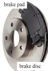
Fig. 2. Structure of disc brake
