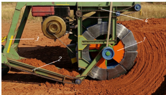
Fig. 2. Testing of a 1540 mm diameter inertial rotor on a field test stand: 1 – driven rotor; 2 – hydraulically driven conveyor; 3 – strain gauge frame; 4 – stand cart
