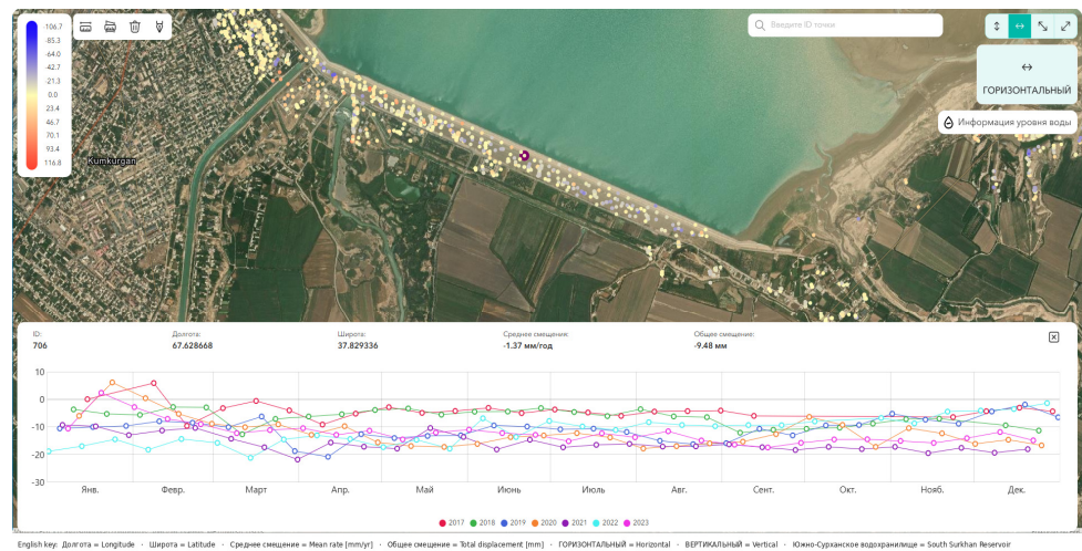
Fig. 20. Point ID 7937, located on the dam, recorded a horizontal displacement of 31.70 mm over the entire observation period
