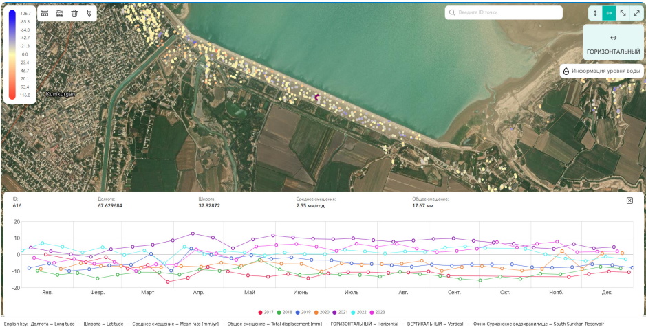
Fig. 22. Point ID 616, located on the dam, recorded a horizontal displacement of 17.48 mm over the entire observation period
