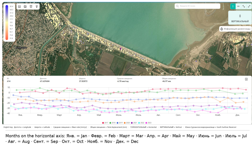
Fig. 27. Point ID 614, located on the dam, recorded a vertical displacement of -6.78 mm over the entire observation period
