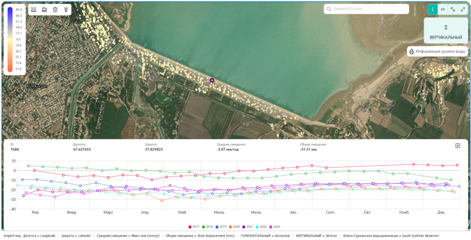
Fig. 24. Point ID 7684, located on the dam, recorded a vertical displacement of –21.31 mm over the entire observation period
