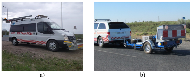
Fig. 1. a) A mobile diagnostic laboratory; b) a falling weight deflectometer. The photographs presented in this paper were taken by the co-author Azamat Zhaisanbayev during field studies carried out in July 2017 on a road section (length: 47 km) of the “Ekaterinburg-Almaty” highway located in the Kostanay region, Kazakhstan
