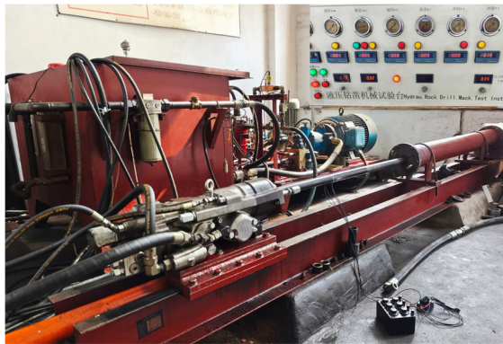
Fig. 5. Hydraulic rock drill impact performance test bench by stress wave method.
