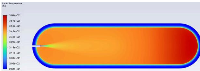
Fig. 8. Static temperature contour showing axial temperature gradient
