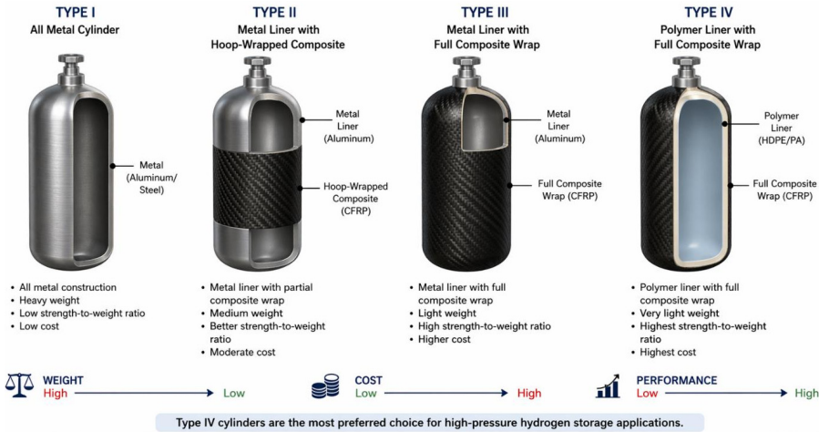
Fig. 1. Types of hydrogen storage cylinders
