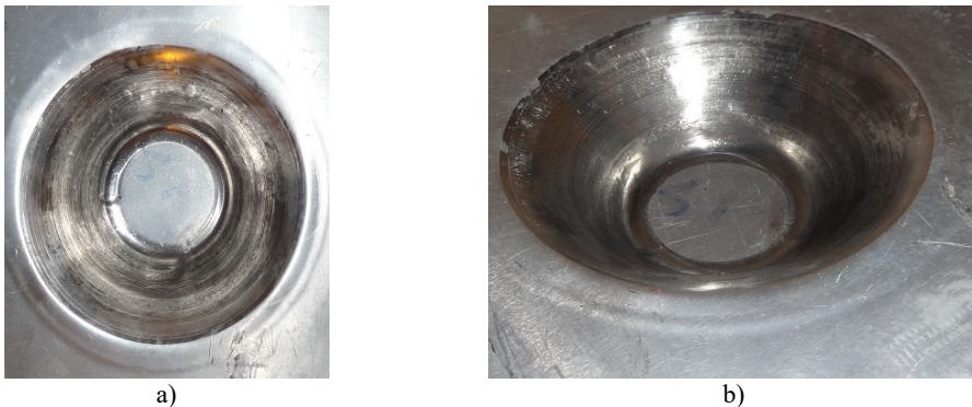
Fig. 7. a) Geometry of the formed hyperbolic part, b) laminated sheet after performing the SPIF process
