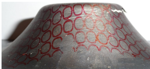
Fig. 8. Deformed circular grid pattern in the necked zone of the formed hyperbolic part, shown across the curved wall
